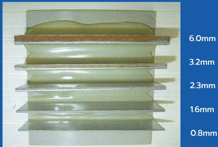
Appearances of cut edge on each thickness of ZAM® after 5 years in coastal environment in Okinawa.
